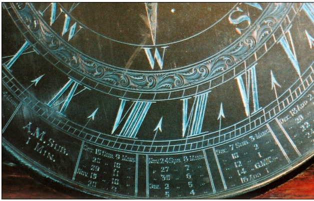
Fig. 4. Close-up of the dialplate showing the time correction ring, the arrowhead half-hour marks and the decorative engraving. Note also the instruction "A.M. Sub. 1 Min." on the left.
